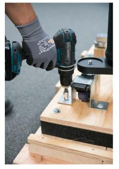
7. USING A 3/8" DRIVE RATCHET OR CORDLESS DRILL WITH A 9/16" SOCKET BIT REMOVE THE 2 BOLTS SECURING THE M2 SHIPPING BARS TO THE CRATE BASE.
