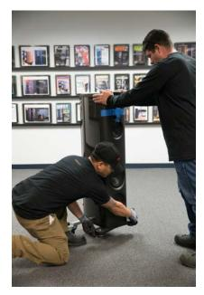
15. WITH A PERSON HOLDING THE FRONT OF THE M2, CAREFULLY TILT THE M2 FOWARD
