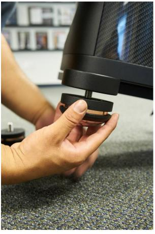
17. TILT SPEAKER FORWARD, UNTHREAD AND REMOVE THE SHIPPING BARS FROM THE BOTTOM OF THE M3. YOU WILL NEED A 3/8" HEX BIT TO REMOVE THE LARGE FASTENER ON THE SHIPPING BAR. YOU WILL NEED TO USE A 5/16" HEX BIT TO REMOVE THE SMALLER SHIPPING BAR FASTENER. INSTALL THE M-POD BY CAREFULLY THREADING IT IN TO POSITION. M-PODS WITH A SHORT STUD MUST ONLY BE INSTALLED IN THE REAR SECTION OF THE STAND. M-PODS WITH LONGER STUDS ARE TO BE INSTALLED IN THE FRONT TWO STAND OUTRIGGERS.
