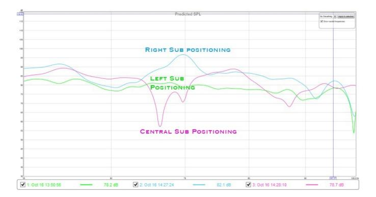
Here you can see for a single subwoofer the Left position rear corner positioning is the best. It is much smoother from 50 - 100 Hz.
