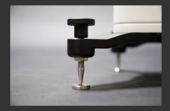
Lift the speaker up and stand it up in the listening position. For hard floors, position floorsavers under 4 spikes. Level speaker by turning adjustable knobs on feet. When leveled, tighten the hex nut to the bottom of the leg which holds the foot.
