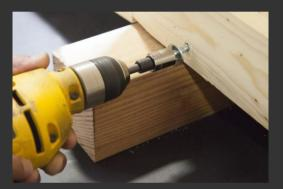
Using a socket wrench or drill with ½" socket bit, remove 8 screws from around the bottom of the crate.
