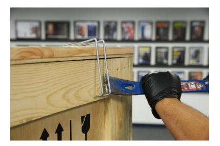
**3.** WITH THE CLAMPS REMOVED, CAREFULLY REMOVE THE CRATE DOOR AND SET IT ASIDE.
