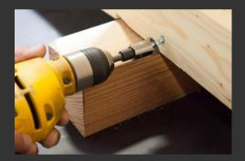
Unfasten 2 x hex bolt screws on the lower front of crate with 9/16" socket wrench. Remove front of crate. Remove Grill from inside of crate. Unfasten 9 x Hex 3" shipping bolt with 9/16 wrench around three sizes of crate.
