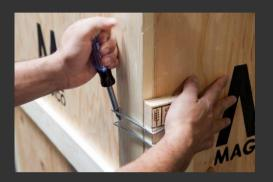
Remove 4x L-shaped clamps from front of crate using a flathead screwdriver.
