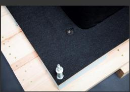
Reach underneath the speaker, and between the foam to unfasten the 3 x Hex bolt  $3/8-16 \times 1-3/4$ " that are attaching the speaker feet to the base of the crate. Carefully tilt the speaker and maneuver the feet out of the cut-always in which they were seated.
