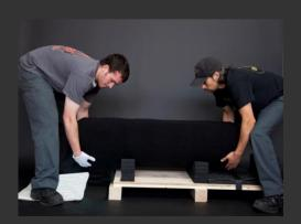
With two people, lift the speaker from the bottom and move the speaker down on the base of the crate until the top of the speaker is lying in the middle foam rib of the crate.
