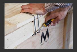
Remove 10 clamps using a flat-head screwdriver or pry bar.
